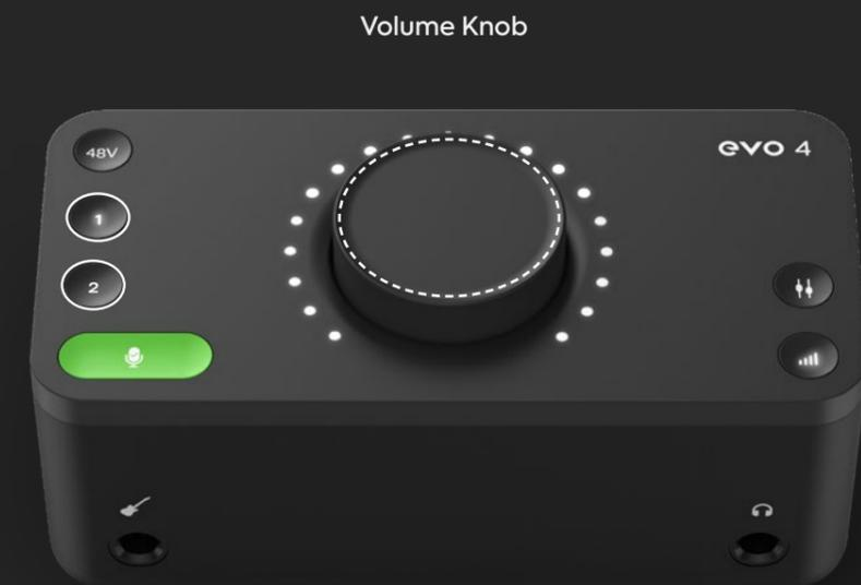
You can manually control this by pressing one of the Input buttons and then turning the Volume Knob. The meters will light up to show you the approximate gain level.
