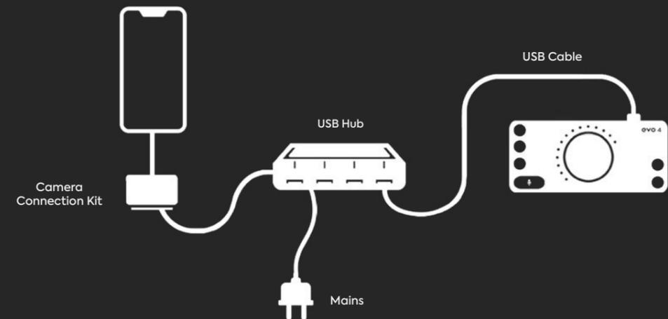
Once connected, the iOS device will automatically use EVO 4 as the sound device. For details on how to setup EVO 4 in recording applications such Cubasis or Auria Pro, please refer to the developers documentation.
