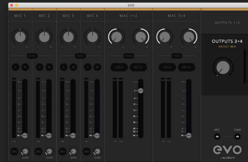
Examples of when you may wish to use this would include, having an engineer using the main speakers (Outputs 1 + 2) and having an artist using headphones (Outputs 3+4) with both listening to separate mixes. The engineer would use the Outputs 1+2 to listen to the overall mix for example while the output 3+4 mix can be used to send a click track or direct monitoring from the microphones just to the artist.
