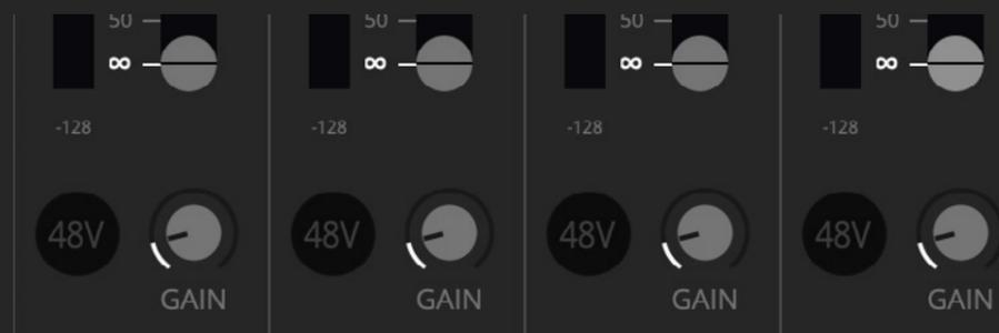
The +48V button will enable phantom power on this channel and the Gain control will adjust the gain level on the EVO 8 itself. Allowing you to make quick changes to your setup without having to look away from the computer during a busy session.
