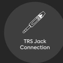
To connect a line-level device, use a 1/4" TRS jack, which will connect to the centre of the Combi connector. The Line input automatically reduces your signal level slightly to minimise the chance of overloading the input and causing distortion.
