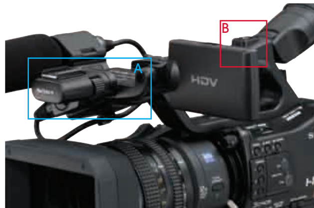
A:Removable Front Shoe B:Screw Hole
