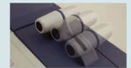
3. T-Bar control of digital video effect transition
